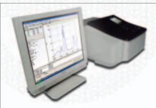
Using the UVProbe software provided makes it possible to control the UV-1800 with a PC. UVProbe is an all-in-one software product that includes the following four functionalities: Spectrum mode, Photometric (quantitation) mode, Kinetics (time-course) mode, and a superb Report Generator.
